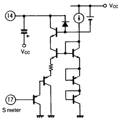
17. Preventing Incorrect RF AGC time-constant switching, Seek Operation
