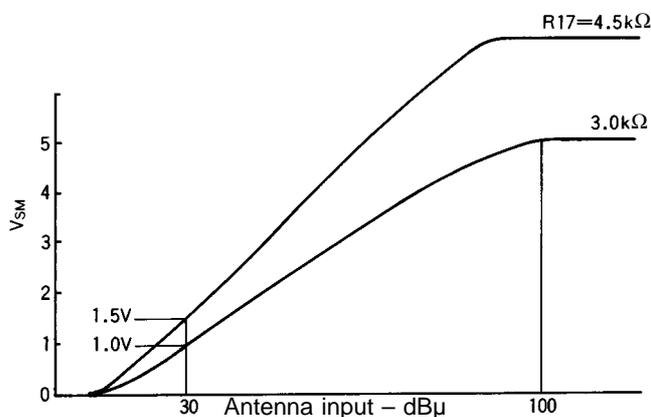
The IF signal from the IF amplifier is detected, on pin 16 the signal that determined the bandwidth characteristics through the narrowband filter BFU450CN (BFU450CN is equivalent to the amplifier emitter load) is detected, and the S-meter output is output by the S-meter drive circuit by driving with current the load on pin 17. Therefore, the S-meter output  $V_{SM}$  on pin 17 has the following relationship with the S-meter load R17.
