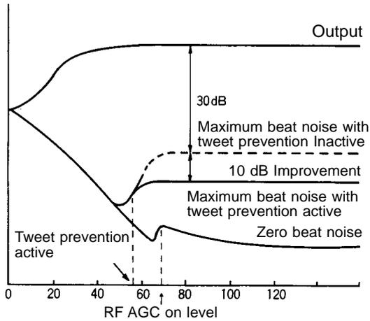
The AGC ON level for  $f_r = 90$  kHz is reduced by 10 dB to reduce the signal level on the varactor diodes. The microcontroller determines when the tuner is receiving at 900 kHz and forces the HIGH-level signal present on pin 18 and SD  $V_{DD}$  to LOW, reducing the ON level by 10 dB. This gives the signal-to-noise characteristics shown below.
