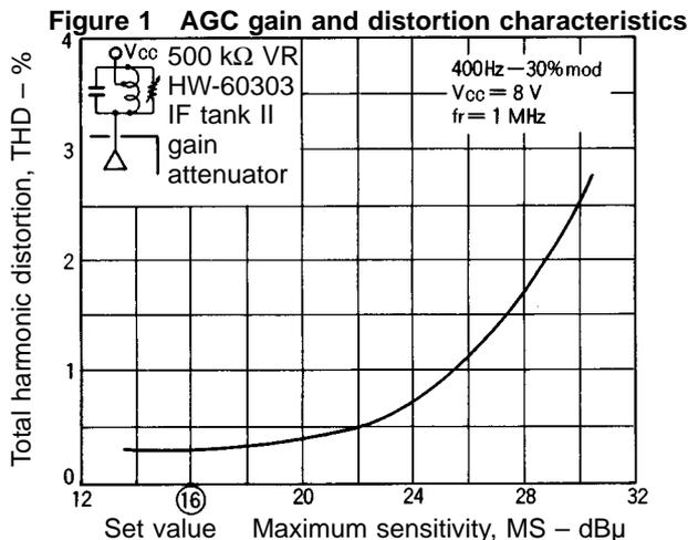
The IF stage block diagram is shown in the figure above. The output current from pin 12 is converted to a voltage and detected by pin 14 of the IF AGC circuit. IF Amplifier I prevents the input signal from exceeding the dynamic range of IF Amplifier II. The relationship between the gain and distortion of the IF stage is shown in Figure 1.
